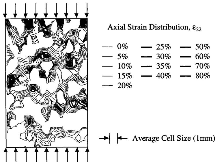
Fig. 9. Axial strain distribution under nominal compressive strain  $\epsilon = 20\%$  (AlMg1Si0.6, transverse orientation,  $\rho^*/\rho_s = 0.25$ , contours with  $\epsilon_{22} > 20\%$  shown in bold). Cuboid specimen geometry.
